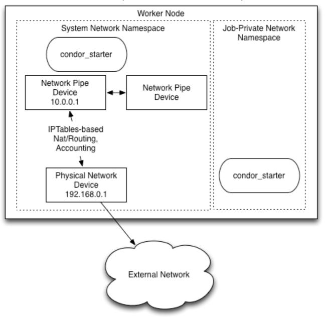
Parent starter passes one end of network pipe to network namespace, Child starter configures routing and IP address
